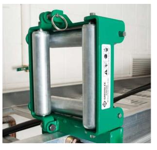
tray type sheaves. A set screw handle locks and unlocks an adjustable sliding leg, eliminating the need to access the top and bottom of the tray to securely attach the sheave. Users can quickly adjust to the appropriate rung spacing on the cable tray with no loose pieces and won't need to purchase separate sized tray sheaves.
